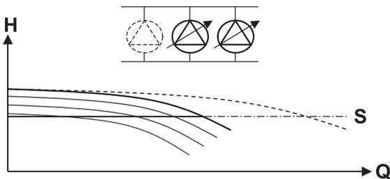
Figure 17: 2 pump operation, 2 pump variable
