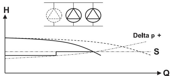
Figure 23: 2-pumps operation
