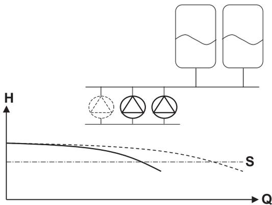
Figure 14: 2 pump operation
