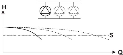
Figure 10: 1 pump operation
