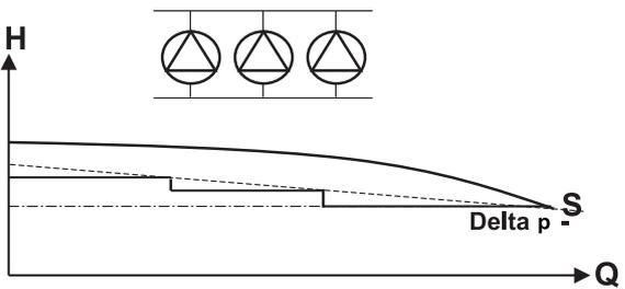
Figure 27: 3-pumps operation
