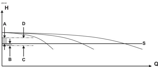
Figure 21: Pressure settings set points variable speed
