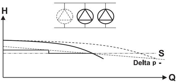
Figure 26: 2-pumps operation
