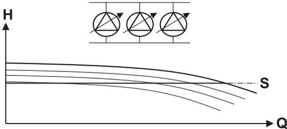
Figure 18: 3 pump operation, 3 pump variable
