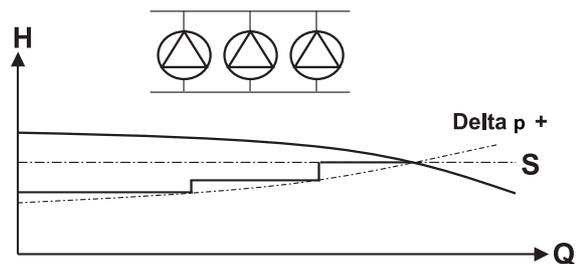
Figure 24: 3-pumps operation
