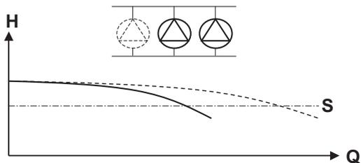
Figure 11: 2 pump operation
