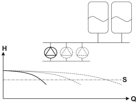
Figure 13: 1 pump operation
