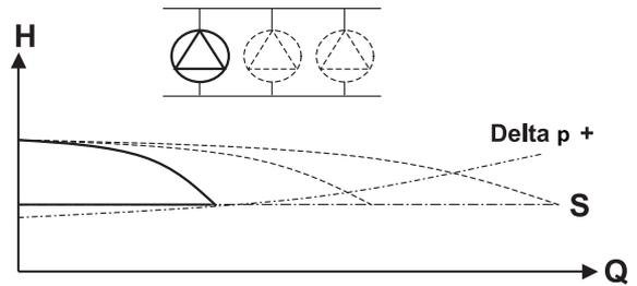
Figure 22: 1-pump operation
