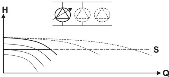
Figure 16: 1 pump operation, 1 pump variable
